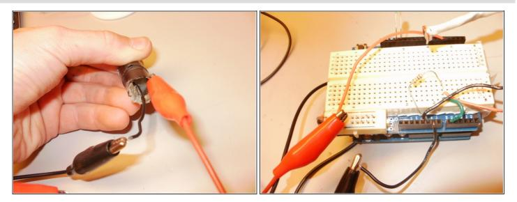
• Remove the end cap and take out the batteries. Inside, there should be a spring, connect one of the alligator clips to this spring. Most laser pointers have a completed circuit when the end cap is on, so connect the other alligator clip to some metal on the actual metal housing of the laser pointer. Connect one of the alligator clips to GND, and the other to digital I/O pin 4. Finally, you can use tape to secure the button down, so the laser pointer is always on.
